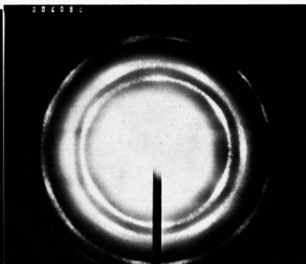
Fig. 3. Electron diffraction pattern taken from a specimen decorated at a substrate temperature of 900^\circ\text{C} .
